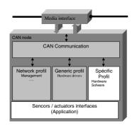
Figure 2. Network node architecture
